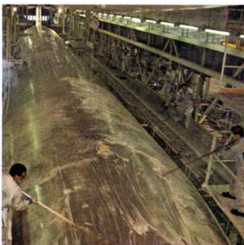
Pantheon's chromium-free PreKote surface pretreatment is applied to a Continental Airlines Boeing 777-200 at HAECO in Hong Kong.
